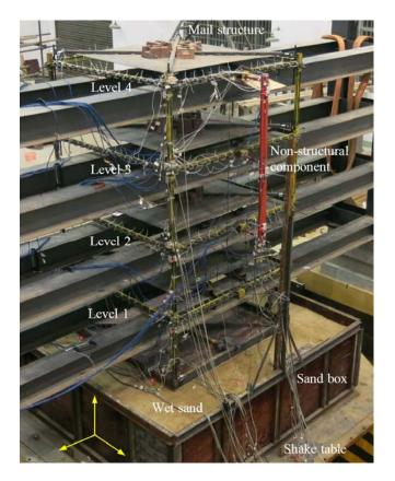
Figure 2. Main structure, non-structural component and sand box on shake table.
