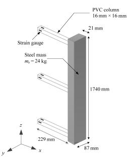
Figure 3. Sketch of the non-structural component.
