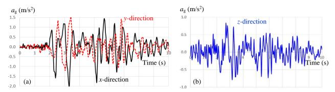
Figure 4. Ground excitation. (a) Horizontal components and (b) vertical component.
